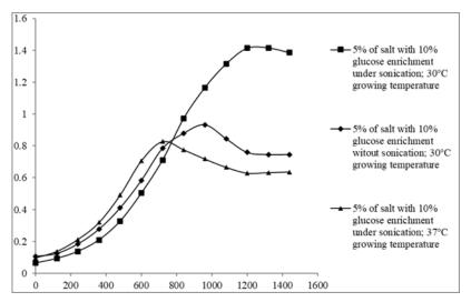
Figure 1. Comparison of sigmoid curves of selected yeast strain B (*Candida* spp.) among the different growing conditions; whereby the sigmoid curves of sonicated yeast in the medium of 5% salt, 10% glucose, and 30°C growing temperature was compared to non-sonicated yeast in the same medium, and the comparison was made between sonicated yeast at 30 and 37°C growing temperatures.
